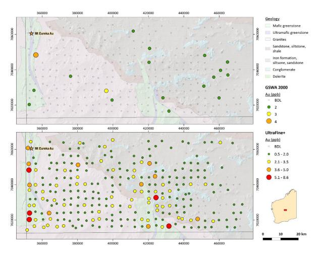
Figure: Gold (ppb) in soils in the Kingston 1:250 0000 map sheet. A) Original GSWA data with only a few detectable Au values, B) the new results of the Ultrafine+ method developed in this MRIWA project using the same samples, clearly showing the vast improvement in Au information. Mt Eureka is the only known small Au deposit in the region (mined in the 1930s). Geology is generalised and based on the data from GSWA (2014).
